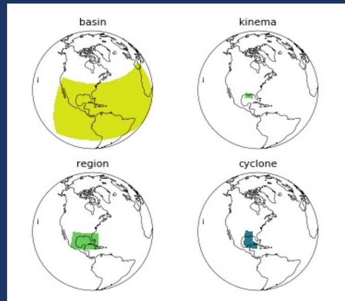
Example of grid domains for multiple independent wind/pressure overlays.
