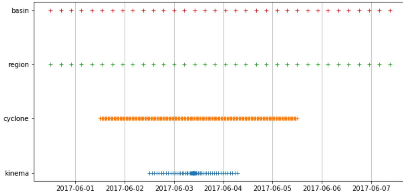
Example of independent time-stepping for each overlay, including individual start/stop and non-regular timestep intervals.
