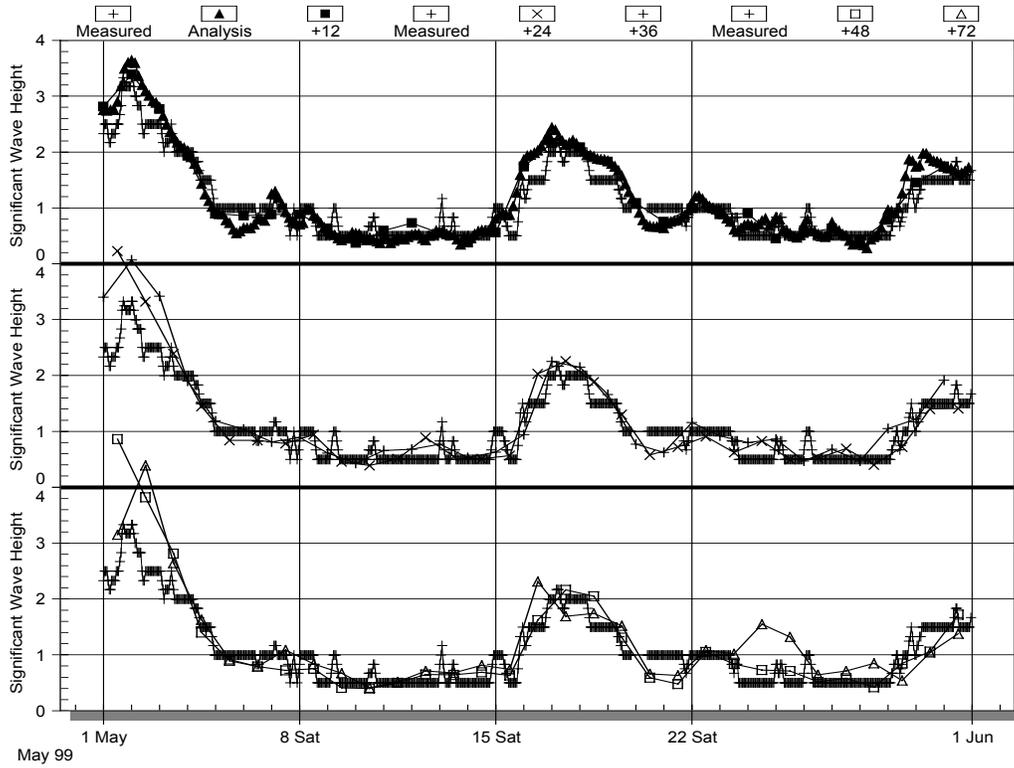
Figure 5. Comparison of model waves at buoy 41009.
